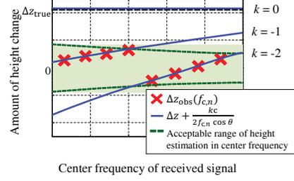
Fig. 2. Fitting approach for height change estimation with multiple frequency bands.
